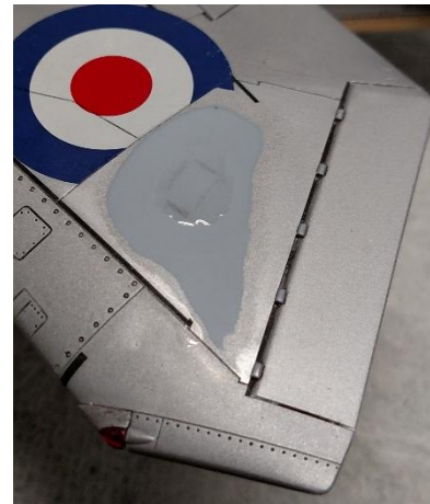
Figure 6 Sanded and polished with a puddle of thin CA glue as filler. The pencil rectangle describes the limits of the divot.
